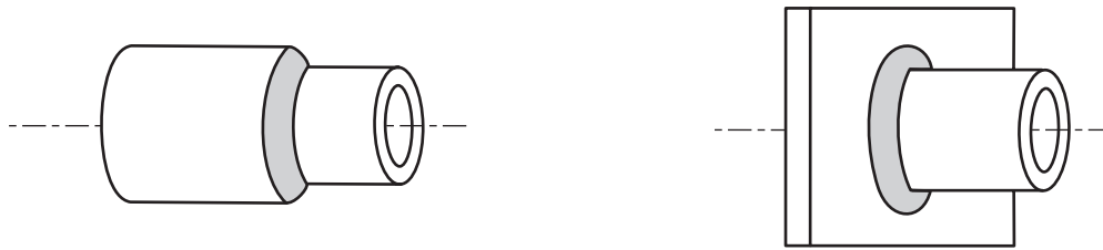
(E) MULTIPLE WELDING TEST POSITION—5F
